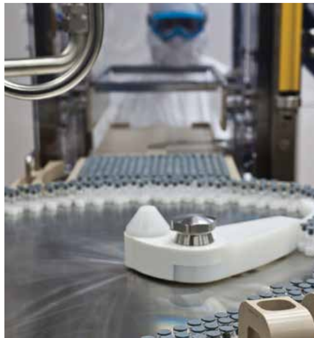
All filling units are integrated in a RABS (restricted access barrier system), which mitigates risk of contamination by minimizing human contact with products during manufacture.
