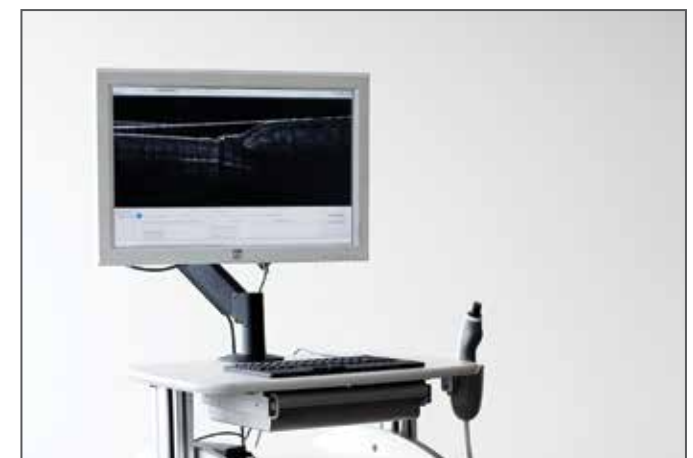
The Diagnostic Photonics Imaging System places a live view of tissue microstructure at the physician's fingertips, providing immediate insight into tissue microstructure.
